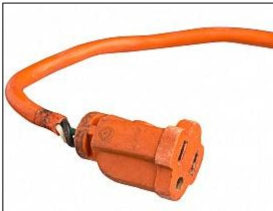
Damaged extension cord. Do not repair, return to tool room for replacement.
