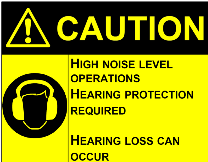
High Noise Level Operation (operation generates noise that exceeds 85 dBA)
